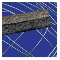
This packing is made from high-quality asbestos yarn, reinforced with stainless steel wire, and closely braided for enhanced durability. Treated with a high-temperature self-lubricant, it offers exceptional performance in steam, butane and propane gases, oil vapor, furnace oil, and more. Known for its anti-corrosive properties, high strength, and durability, this packing is the ideal choice for demanding industrial environments.
