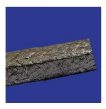
Cotton Graphited and Lubricated Gland Packing is an economical and versatile solution made from high-quality natural cotton fibre yarn. It is densely braided and impregnated with graphite and mineral lubricants, providing thorough and long-lasting lubrication that minimizes shaft friction and wear. The flexible yet robust nature of this packing makes it ideal for rotating pumps, reciprocating pumps, and valves handling fresh water.
